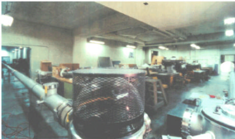
Figure 5. The test system used: the 40-m beam-tube at the right-hand side of the photograph houses the interferometer experiments outlined here.
