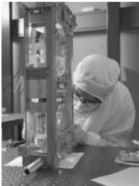
Figure 1. Intermediate mass on top and mirror at the bottom clamped in a steel frame. On first plane ears bonded on both the masses and two fibres welded.
